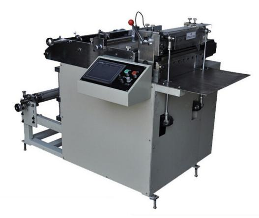
The machine uses micro-computer system, under knife fixed, the upper knife up and down movement for precise cutting, can track the printing mark or can also set the length for the sheet cutting.
